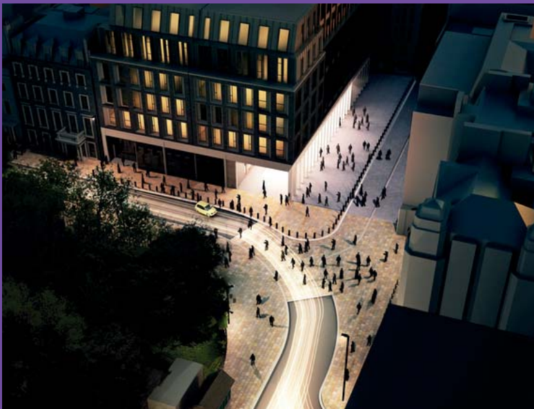
Crossrail Bond Street, London – The site design enforces speed reduction for vehicles approaching the station and bollards are placed to create the stand-off distance.
